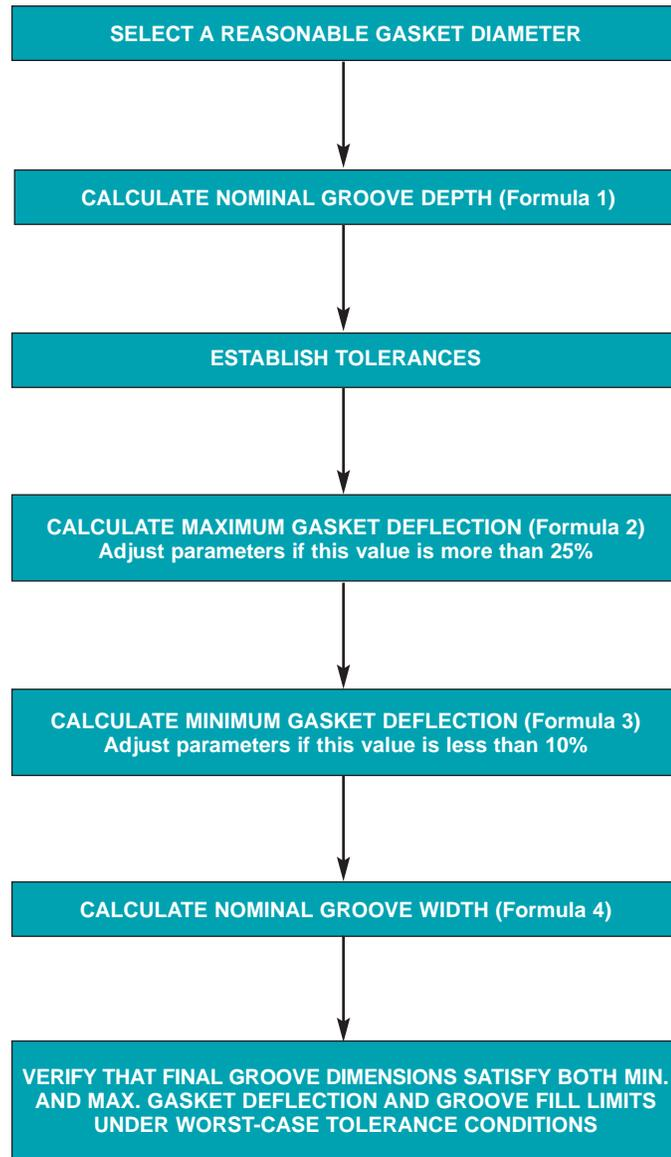
Figure 29 Procedure for Calculating Gasket and Groove Dimensions
