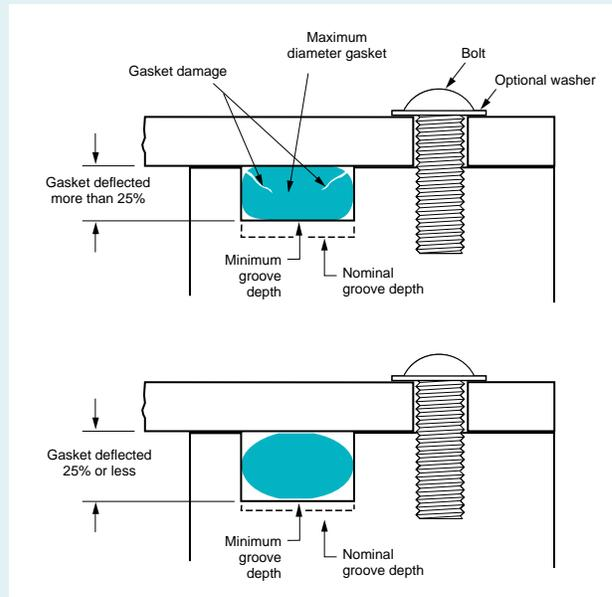
**Figure 28e** Section B-B from Figure 28c – Worst Case Maximum Groove Fill (*Maximum gasket diameter in minimum groove depth and width*)
