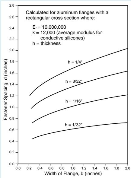
Figure 24 Fastener Spacing
