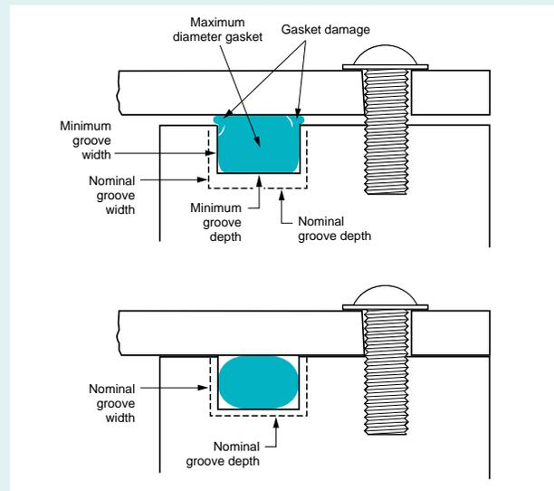
**Figure 28f** Section C-C from Figure 28c – Worst Case Minimum Deflection (*Minimum gasket diameter in maximum depth groove, aggravated by cover bowing and lack of conformity between mating surfaces*)
