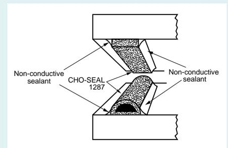
**Figure 16** “Seal-to-seal” design incorporating CHO-SEAL® 1287 conductive silver-aluminum fluorosilicone gaskets on both mating flange surfaces. Gaskets are bonded and edge sealed to prevent moisture from entering the gasket/flange area.
