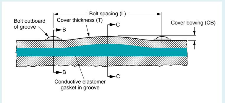
**Figure 28d** Section B-B from Figure 28c – Worst Case Maximum Deflection (*Maximum gasket diameter, minimum groove depth*)
