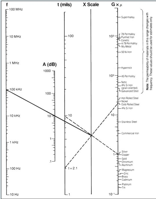
Figure 6 Absorption Loss Nomograph<sup>1</sup>
