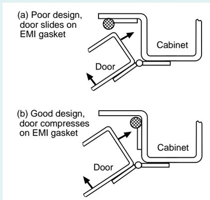
**Figure 34 a-b** Sliding Motion vs. Straight Compression
