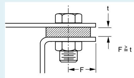
**Figure 12** Flat Gasket on Sheet Metal Flange
