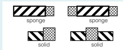
**Figure 37** Normal and High Pressure COMBO STRIP Gaskets
