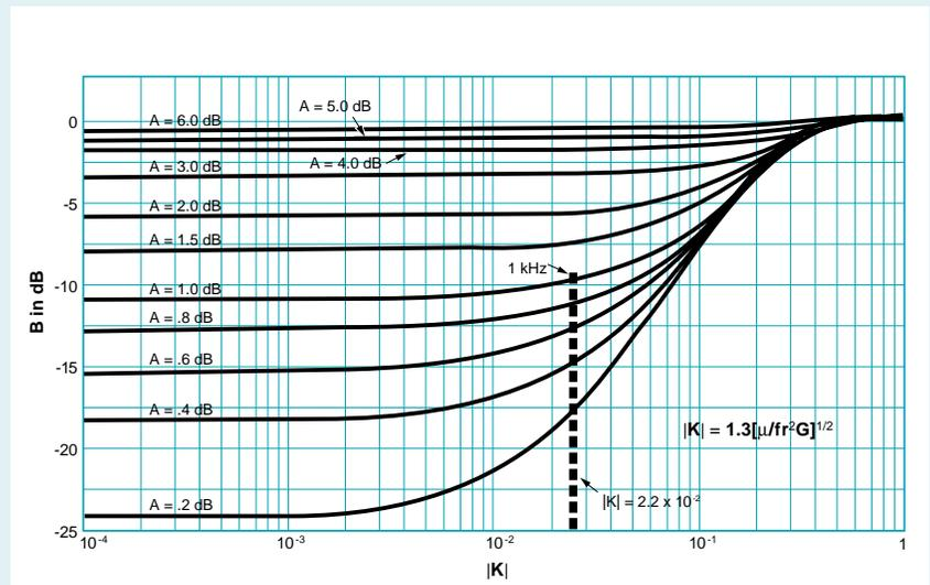
Figure 9 Solving for Secondary Reflection Loss (B)<sup>1</sup>
