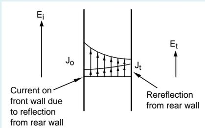
**Figure 3** Variation of Current Density with Thickness for Electrically Thin Wall enclosure, the current distribution in the gasket will also be the same assuming it could perfectly fill the slot. (This is not possible due to mechanical considerations.)
