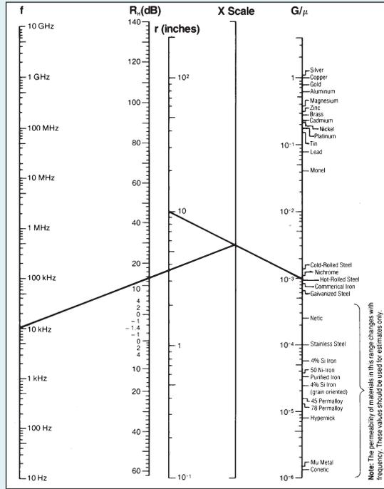
Figure 7 Magnetic Field Reflection Loss Nomograph,  $R_H$ <sup>1</sup>
