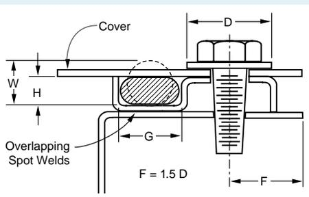
**Figure 11a** Shaped Sheet Metal Container
