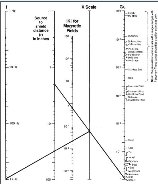
Figure 8 Magnetic Field Secondary Reflection Loss Factor Nomograph<sup>1</sup>
