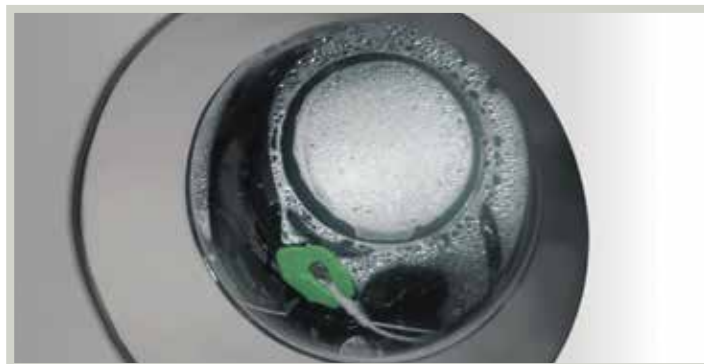
Figure 1: Desiccant could not prevent severe condensation from forming and becoming trapped within this sealed enclosure.
