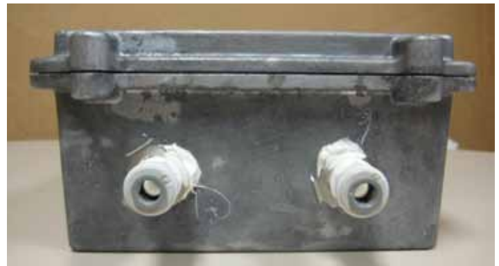
FIGURE 2: ALUMINUM HOUSING WITH PORTS INSTALLED FOR PRESSURE AND TEMPERATURE PROBES
