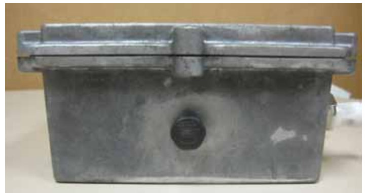
FIGURE 3: ALUMINUM HOUSING WITH GORE® PROTECTIVE VENT INSTALLED
